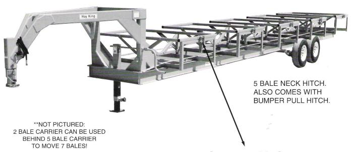
Balanced Saddle Units dump one bale at a time with easy operating spring release pin.
